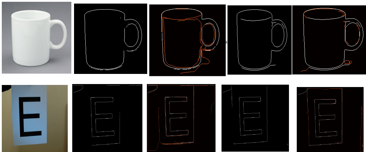
Figure 5. In-door test images. First row shows an original cup and its edges obtained by Sobel, Sobel+RES, Canny, Canny+RES respectively. The second row is the photo of a big letter 'E' on a paper, and its edges as in the first row. RES not only extends the unfound/missing edges but also fills the gap between the disjoint edges and completes the contour continuity.
